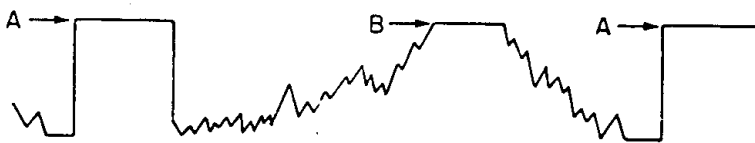
Figure 5—Overloaded or Clipped Video and Sync Signal.
