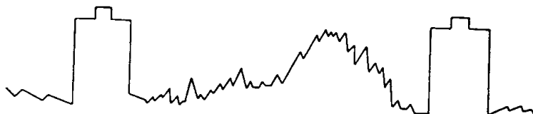
Figure 4—Normal Video and Sync Signal.
